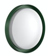
LED source included. Integrated power supply 220-240V ON/OFF and dimmable 1-10V or DALI. With IP65 cable guide for rubber cables 5mm<ø<10mm and a 2-pole connection box for a fast connection. To ensure the tightness of the cable guide it's recommended to use flexible electric cables suitable for exterior use.
